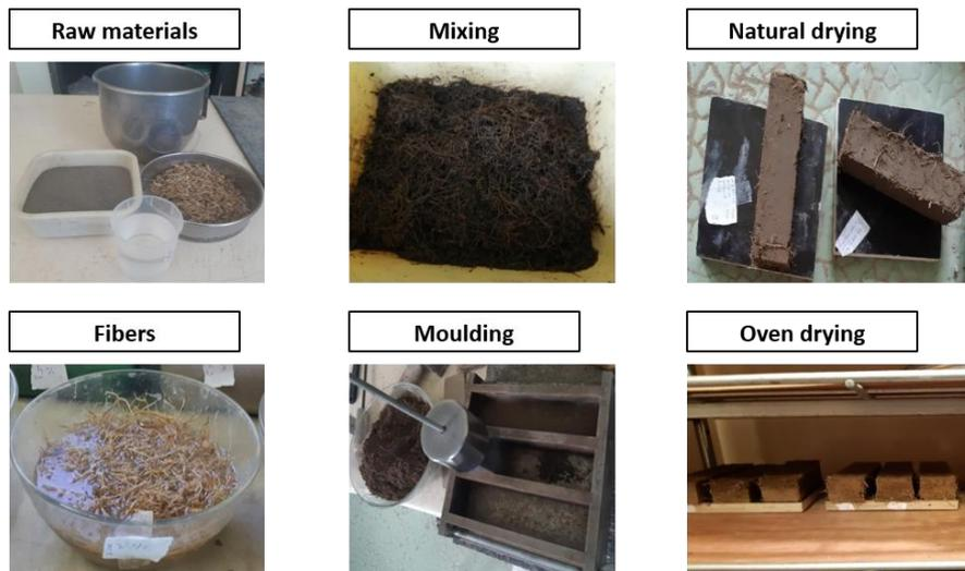
**Figure 1:** Raw material and manufacturing of crude bricks
