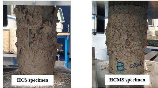
Fig. 3. Shapes of specimen submitted to compressive test, after 50 aging cycles
