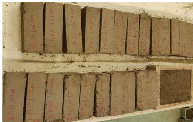
**Figure 2:** Crude bricks samples at different fibers percentage with G-2cm and G-3cm fibers
